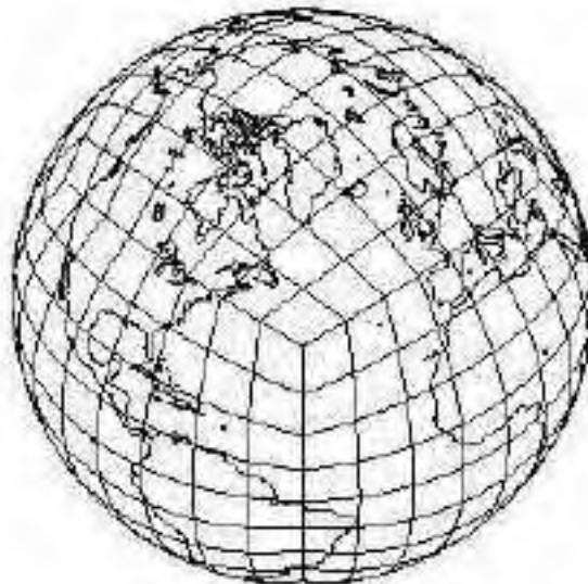
Figure 4.2: Spectral elements method: implemented by means of the "cubed sphere".
